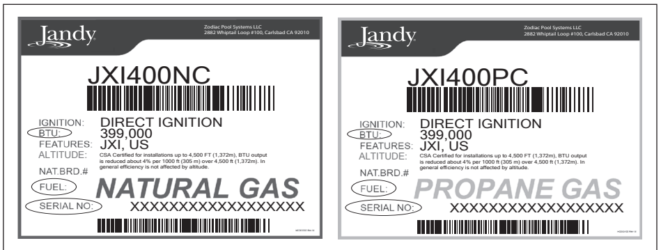
Figure 35. Carton Label BTU, Fuel Type, and Serial Number
